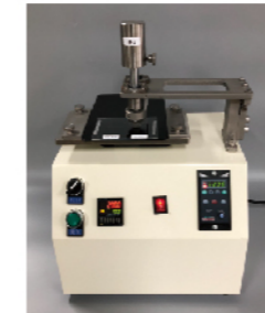
钢丝绒耐磨测试机 Steel wool test machine
